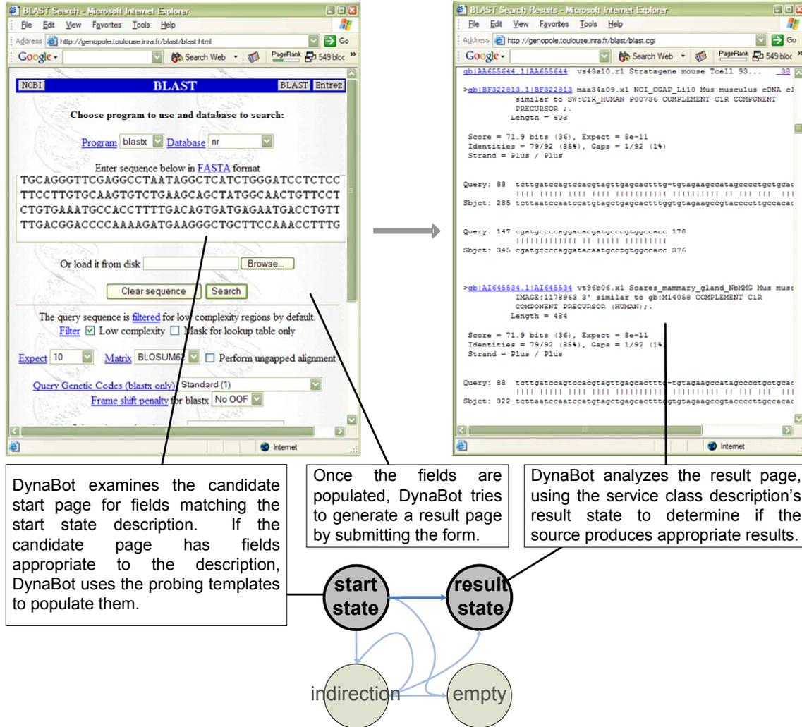
Figure 7: DynaBot Analysis of a Matching Web Source
