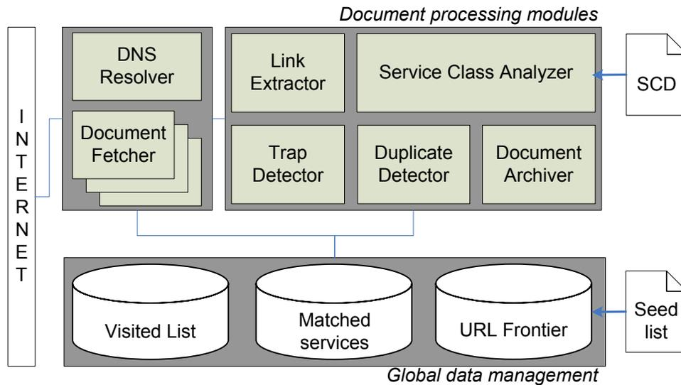
Figure 5: DynaBot System Architecture
