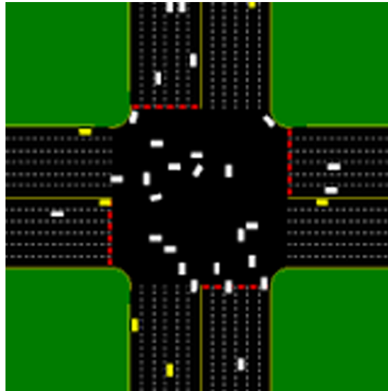
Fig. 6. The AIM simulator depicting a reservation-based intersection in operation.
