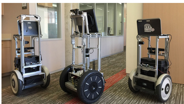
Fig. 1 Three of our Segway-based mobile robot platforms
