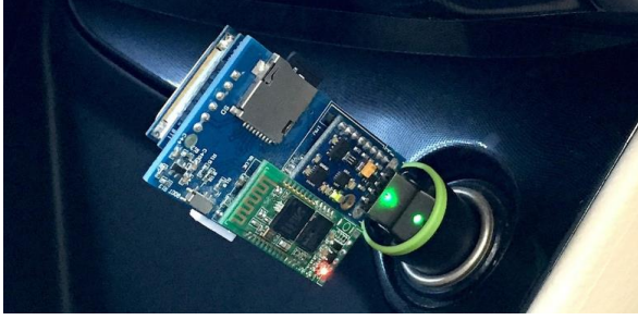
Figure 6.8 IMU Device Installed in a Vehicle, with Power Supplied through a USB Car Charger
