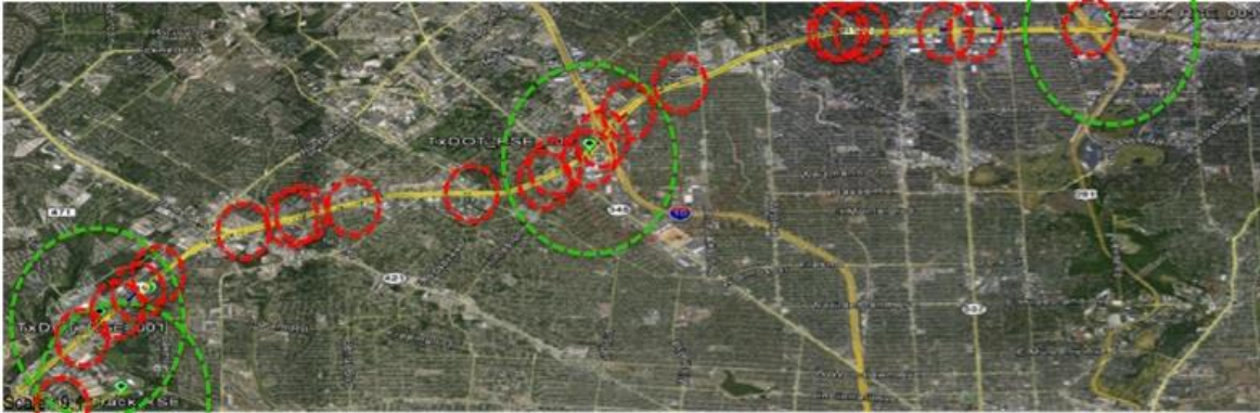
Figure 5.10 Simulated CVs along I-410 in San Antonio Showing Potential for Message Propagation between RSUs
