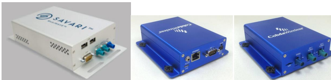
Figure 3.3 OBE DSRC Vehicle Devices Manufactured by Savari and Cohda Wireless
