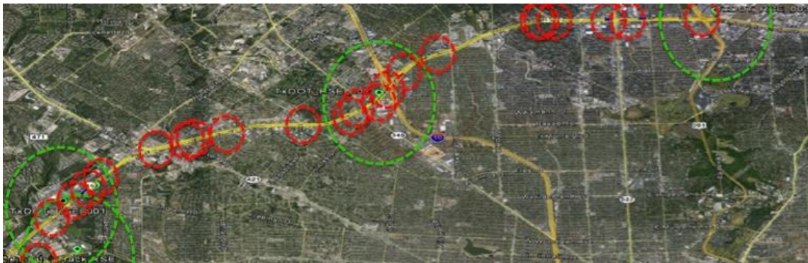
Figure 3.8 Simulated CVs along I-410 in San Antonio Showing Potential for Message Propagation Between RSUs
