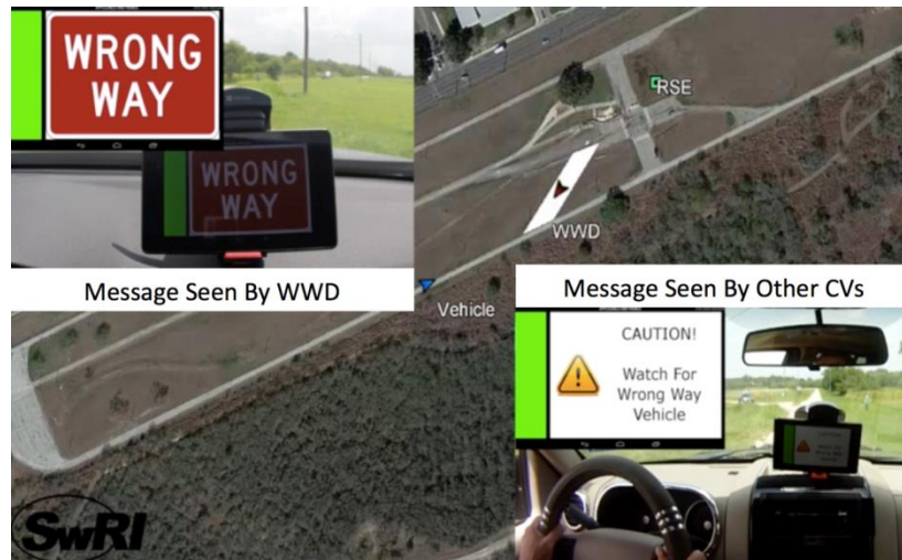
Figure 3.7 CV WWD Messages Sent by RSU
