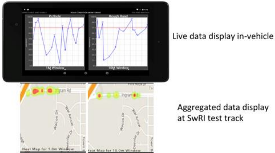
Figure 5.23 Road Condition Monitoring Tablet and Heat Map Displays
