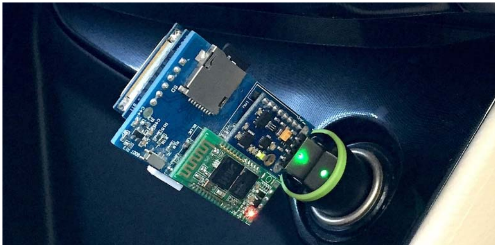
Figure 11.8: IMU Device Installed in a Vehicle, with Power Supplied through a USB Car Charger
