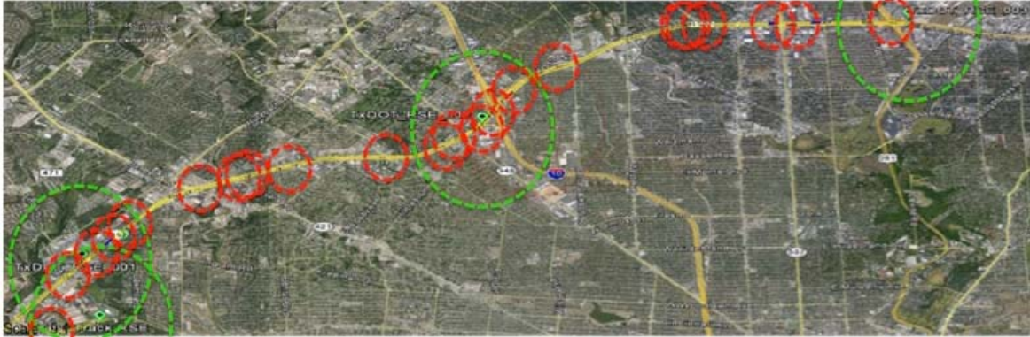
Figure 10.11: Simulated CVs along I-410 in San Antonio Showing Potential for Message Propagation between RSEs
