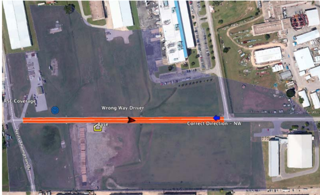
Figure 10.19: Winter Demonstration Venue Showing Effective RSE Coverage Area, Viewing Area, and CV Vehicles During a Demonstration
