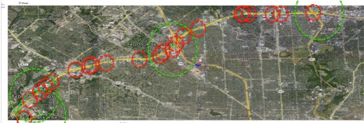
Figure 13.10: Simulated CVs along I-410 in San Antonio Showing Potential for Message Propagation Between RSEs
