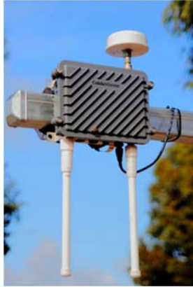
Figure 13.2: RSE DSRC Roadside Device Manufactured by Coda Wireless
