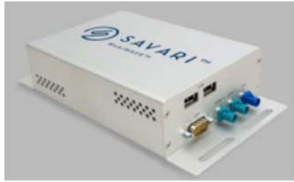
Figure 13.5: OBE DSRC Vehicle Devices Manufactured by Savari
