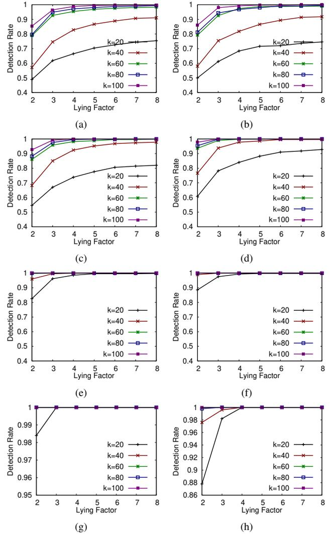
**Fig. 6: PDT's Detection Rate when the ratio of the compromised links: (a) 16.6% ( $\frac{1}{6}$ ). (b) 20% ( $\frac{1}{5}$ ). (c) 25% ( $\frac{1}{4}$ ). (d) 33% ( $\frac{2}{6}$ ). (e) 40% ( $\frac{2}{5}$ ). (f) 50% ( $\frac{3}{6}$ ). (g) 60% ( $\frac{3}{5}$ ). (h) HDT's Detection Rate.**
