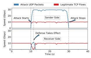
Fig. 14: Throughput restoration for legitimate flows.
