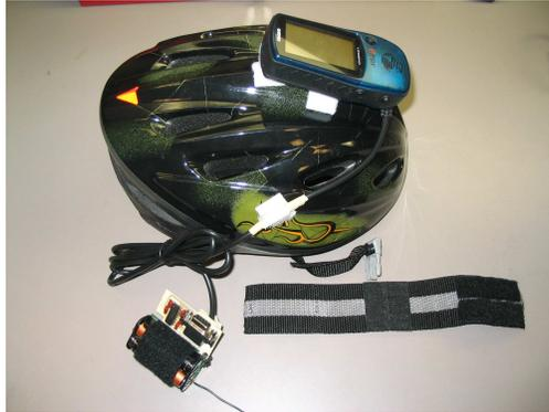
Fig. 4. GPS Mote Assembly
