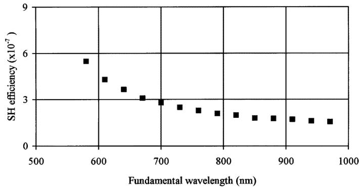
Figure 3. SH beam efficiency plotted against the fundamental wavelength.
