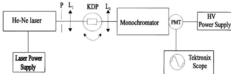
Figure 4. The experimental set-up.
