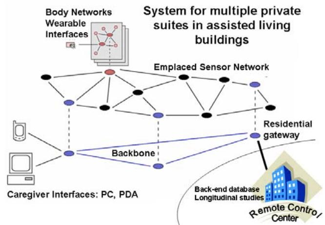
Figure 2: Multi-tiered system architecture, showing physical connectivity.
