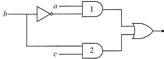
In the diagram above, the inverter and the *AND*-gates labeled 1 and 2 have delays of 9, 10, and 12 nanoseconds, respectively. Wire delays are negligible. For certain values of *a* and *c*, together with a certain transition of *b*, a glitch (spurious output) is generated for a short time, after which the output assumes its correct value. The duration of the glitch is
